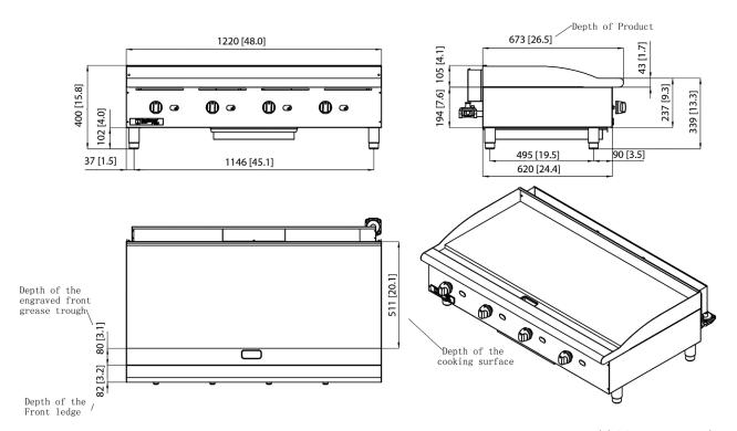
model GCP48 represented measurements in mm [inches]
